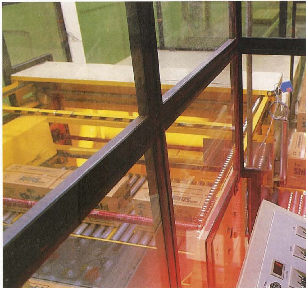
Right: The toilet soaps automatic palletiser is part of a major investment in new technology at the Lever Brothers factory in Port Sunlight
