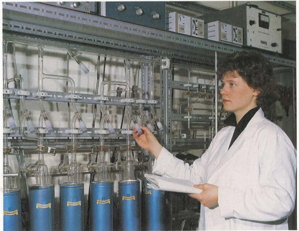
Experimental work on catalysts, which are vital for hydrogenation (fat hardening) in the soap and margarine industries, shown here in the Unilever Research Laboratory at Vlaardingen in the Netherlands
